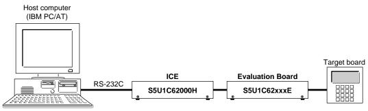
Fig. 2.2.1 System connection diagram
